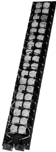
Fig.3. Cylindrical electrostatic loudspeaker. Each strip carries the full frequency range and the sections are coupled to form an electrical transmission line. The inductor assembly is shown below.
