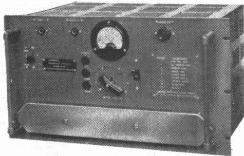
New Ekco ground-to-air v.h.f. transmitter, Type CE91.
