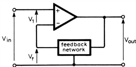
by a factor  $|1 + A_i \beta_i|$ . This factor we now evaluate for an amplifier with a loop gain of 10 ( $|A_i \beta_i| = 10$ ).
