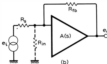
In its mode of use ( $E_1$  short circuited) the source resistance is  $R_s // R_{fb}$  and the noise current of  $R_s$  is significant. Certainly a 47k $\Omega$  source resistor will generate a noise voltage of 3.9 $\mu$ V and provided the input is short circuited this will be shown in the amplifier noise performance.
