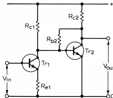
Fig. 10. Skeleton form of two-stage voltage amplifier.
