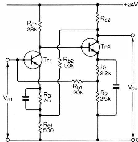
Fig. 11. More detailed version of the circuit in Fig. 10, designed for a voltage gain of 100. [www.keith-snook.info](http://www.keith-snook.info)
