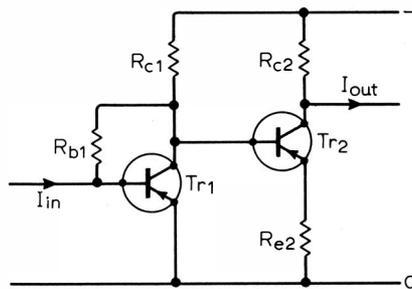
Fig. 8. Skeleton form of two-stage current amplifier.
