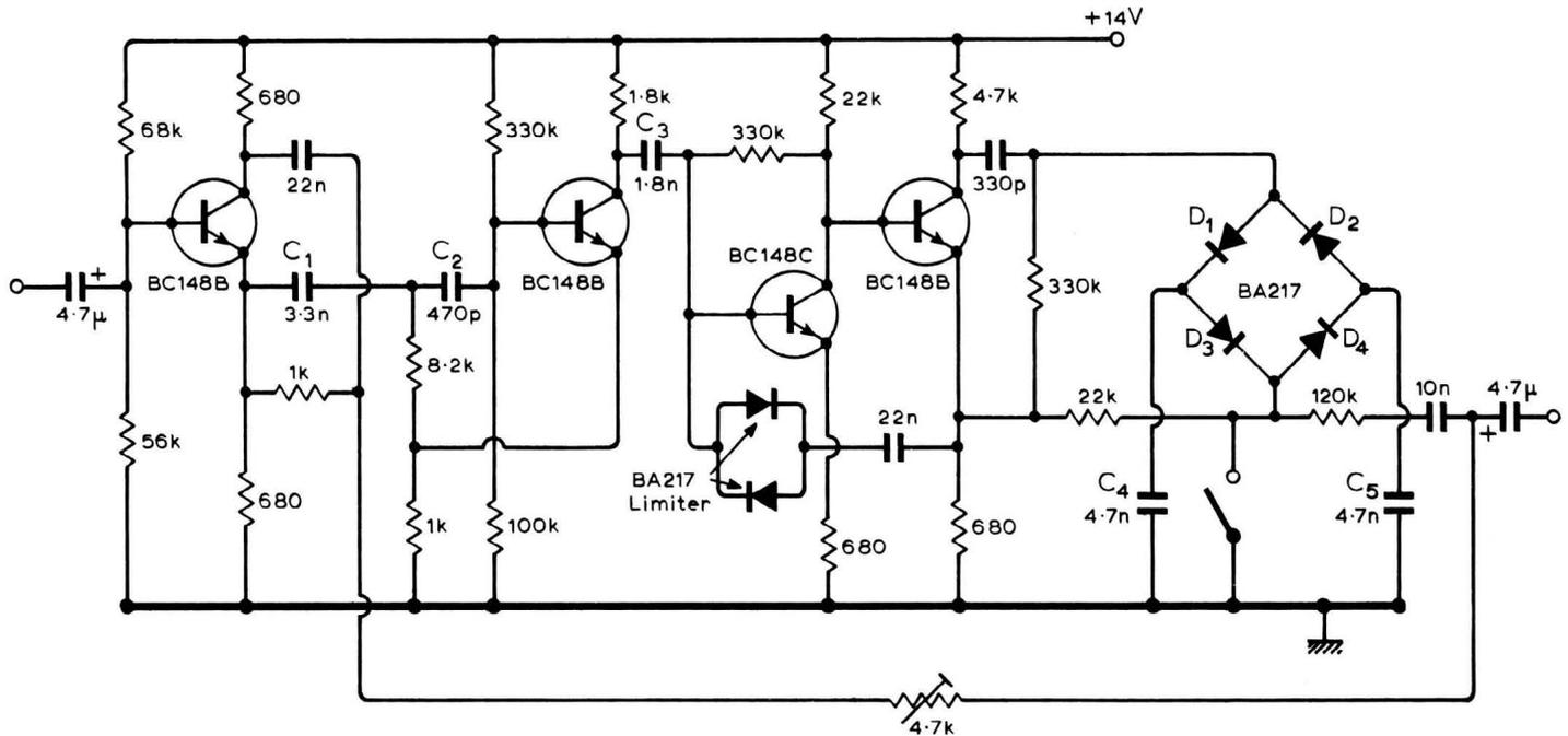
Fig. 2. Complete circuit of Philips dynamic noise reducer. Capacitors  $C_1$ ,  $C_2$  and  $C_3$  form part of the high-pass filter. Diodes  $D_1$  and  $D_2$  and capacitors  $C_4$  and  $C_5$  form a peak detector providing a control potential to attenuator diodes  $D_3$  and  $D_4$ .
