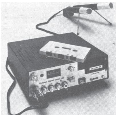
reversing. Low-level amplitude response extends to 12.5kHz (3dB down). Signal-to-noise ratio is quoted as 48dB DIN weighting and 58dB A-curve. Wow and flutter amounts to 0.17% peak. The recorder includes a built-in capacitor microphone with a polarizing potential of only 5V. Power supply can be lead-acid battery, nickel-cadmium battery or from the mains. Price is £182. U.K. agents: Bosch Ltd, P.O. Box 166, Rhodes Way, Watford WD2 4LB, Herts.
