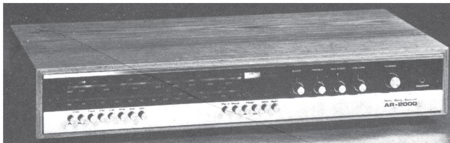
in the r.f. section and new integrated circuits and ceramic filters in the i.f. amplifier. The stereo decoder uses a single i.c. Kit price is about £90 plus £7 for a teak cabinet. Heath (Gloucester) Ltd, Bristol Road, Gloucester GL2 6EE.
