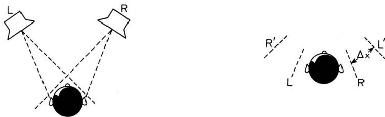
Fig. 6. (left). The effect of crossed soundpaths. Fig. 7 (right). Units put in parallel to simulate crossed soundpaths.
