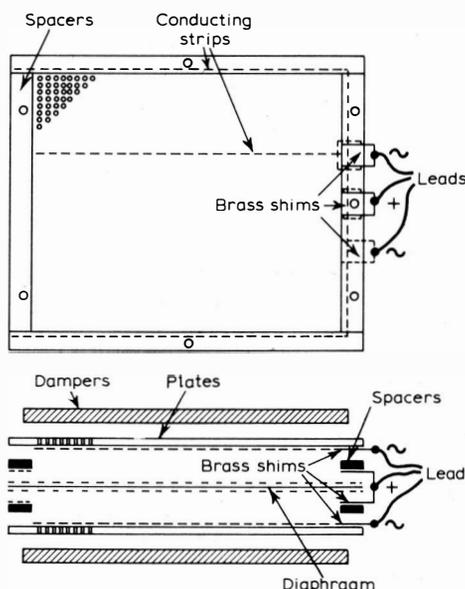
the diaphragm at low frequencies.<sup>2</sup> The high frequency roll-off is well above the audible limit for diaphragm materials commonly used in electrostatic speakers. At certain low frequency the entrained mass of air and the tension of the diaphragm form a resonant system.<sup>1</sup> This resonance determines the lower frequency limit of the device. It should not be made lower than required because this would limit the apparent sensitivity.<sup>2</sup>
