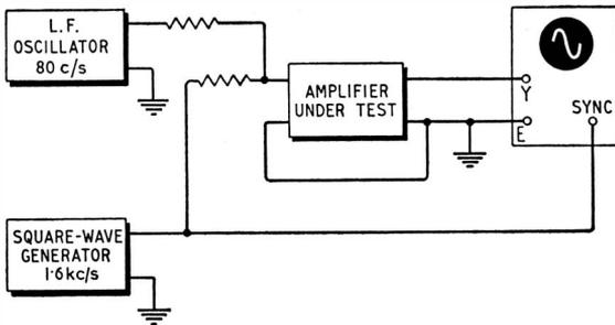
Fig. 1 Test set-up for an audio amplifier.
