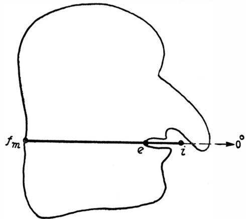
Fig. 6. This kind of Nyquist diagram, in which the oscillation point  $i$  is not enclosed, but which crosses the  $0^\circ$  axis beyond it indicates what is called conditional stability. Some Nyquist lines have very strange shapes.
