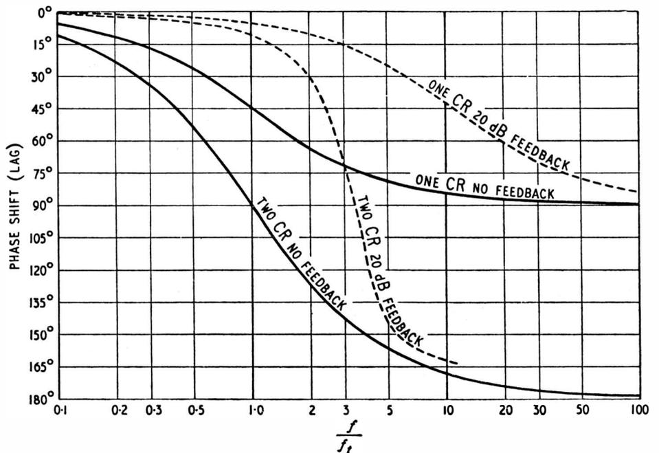
Fig. 4. Phase shift graphs corresponding to Fig. 3.
