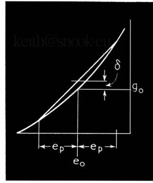
Fig. 4. The sag of a curved characteristic is a measure of the third harmonic distortion.
