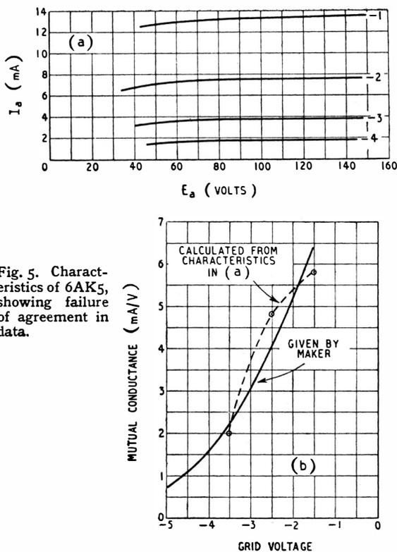
Fig. 5. Characteristics of 6AK5, showing failure of agreement in data.
