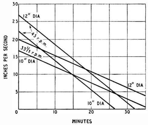
Right : Fig. 8. Data for 10in and 12in discs replotted from Fig. 7 with zero time at start of outer groove.
