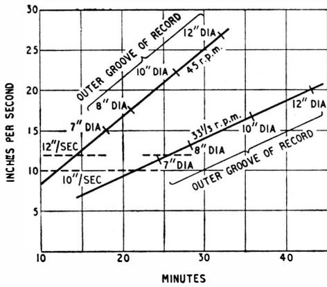
Left : Fig. 7. Groove speed as a function of time, with zero time at the centre of the record.
