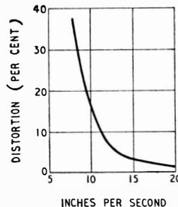
Left: Fig. 4. For a given stylus radius and lateral velocity of cut, distortion is inversely proportional to the fourth power of the tangential (linear) groove speed.
