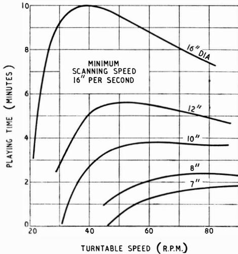
Fig. 1. For a given minimum groove speed there is an optimum turntable speed for maximum playing time with any given outside diameter of record.
