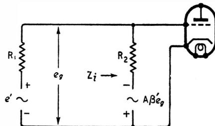
Fig. 3. (right) Illustrating the basic parallel-connected feedback stage.
