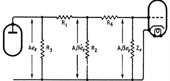
Fig. 6. This diagram is used to show the distinction between distortion reduction and gain reduction factors.
