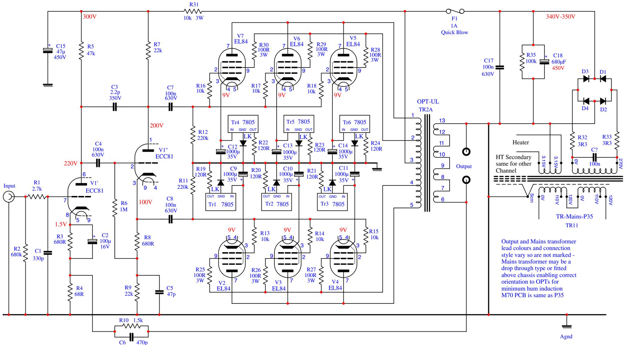
Output and Mains transformer lead colours and connection style vary so are not marked - Mains transformer may be a drop through type or fitted above chassis enabling correct orientation to OPTs for minimum hum induction M70 PCB is same as P35
